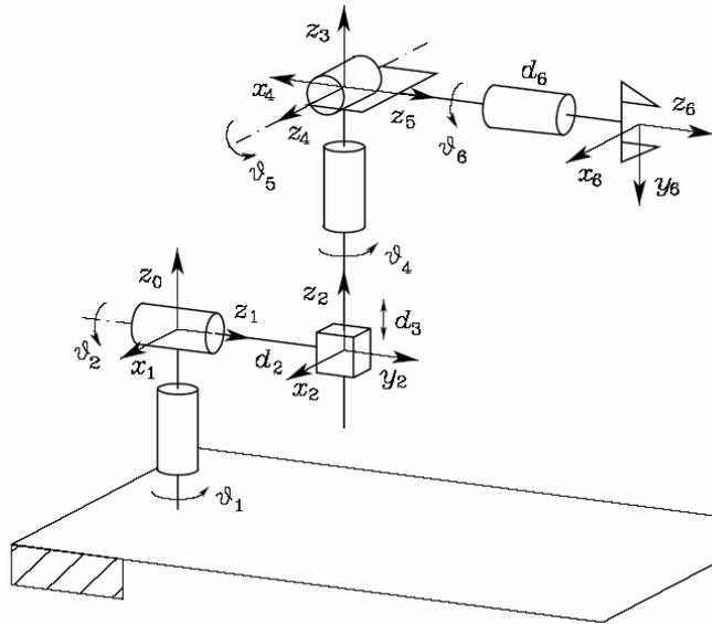
$$J(q) = \begin{bmatrix} z_0 \times (p - p_0) & z_1 \times (p - p_1) & z_2 \\ z_0 & z_1 & \mathbf{0} \\ z_3 \times (p - p_3) & z_4 \times (p - p_4) & z_5 \times (p - p_5) \\ z_3 & z_4 & z_5 \end{bmatrix}$$
