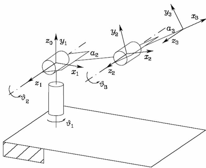
$$J(q) = \begin{bmatrix} z_0 \times (p - p_0) & z_1 \times (p - p_1) & z_2 \times (p - p_2) \\ z_0 & z_1 & z_2 \end{bmatrix}$$
