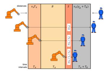
4. Consider now a robot that is compliant with the power and force limiting safety standards. Making reference to the following picture, derive the expression of the maximum value of the relative velocity between robot and human requested by such standard.
