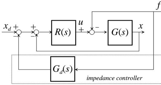
**4.3** Sketch the block diagram of an implicit force control scheme for a single d.o.f. system, in contact with an environment.
