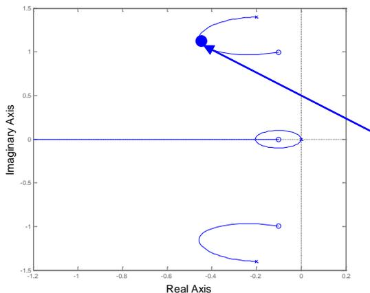
The graphical method consists in selecting the gain of the speed controller in such a way that the damping of the complex and conjugate poles is maximized (see the picture).
