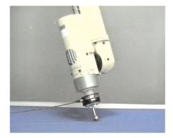
Assume a point contact and draw a contact frame directly on the picture. Based on this frame and neglecting angular velocities and moments, express the natural and the artificial constraints for this problem, and specify the selection matrix.
