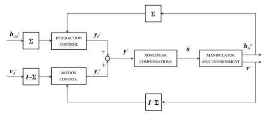
**4.4** Suppose now that along the force controlled direction an explicit force controller has to be designed. Determine the expression of such controller, taking a bandwidth of 30 rad/s.
