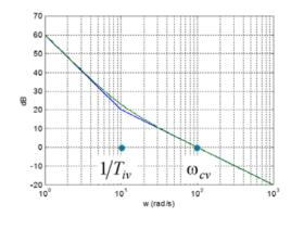
The zero of the controller can be placed in a sufficiently lower frequency range with respect to  $\omega_{cv}$ :
