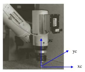
**4.1** Assume a point contact and draw a contact frame directly on the picture. Based on this frame and neglecting angular velocities and moments, express the natural and the artificial constraints for this problem.
