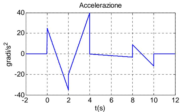
$$\begin{array}{ccccc} t_1 = 0 & t_2 = 2 & t_3 = 4 & t_4 = 8 & t_5 = 10 \\ q_1 = 10^\circ & q_2 = 20^\circ & q_3 = 0^\circ & q_4 = 30^\circ & q_5 = 40^\circ \\ \dot{q}_1 = 0^\circ/s & \dot{q}_2 = -10^\circ/s & \dot{q}_3 = 10^\circ/s & \dot{q}_4 = 3^\circ/s & \dot{q}_5 = 0^\circ/s \end{array}$$
