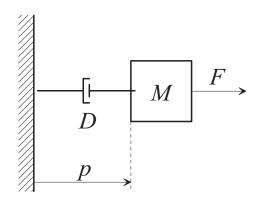
The system is composed by a body of mass M subjected to a viscous friction force, proportional to the speed through the coefficient D.
