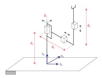
Find the expression of the direct kinematics of the robot, in terms of the position coordinates of the end effector with respect to the joint variables  $\vartheta_1$ ,  $d_2$ , and  $d_3$ .
