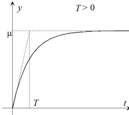
The steady state is reached after approximately 5 times the time constant  $T$ , i.e. after 3.75s.
