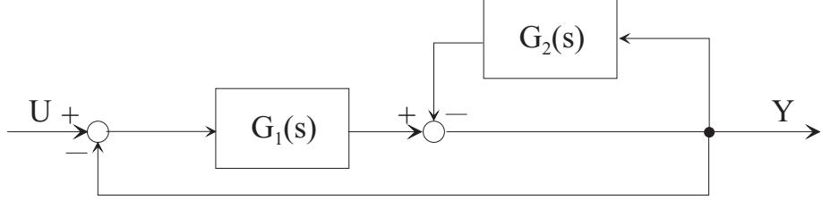
Solve the block diagram by determining the transfer function from  $u$  to  $y$ .
