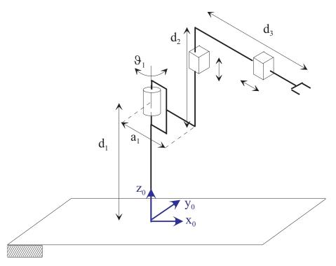
1. Find the expression of the direct kinematics of the robot, in terms of the position coordinates of the end effector with respect to the joint variables  $\vartheta_1$ ,  $d_2$ , and  $d_3$ .
