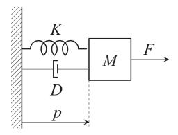
The system is composed by a body of mass M subjected to a viscous friction force, proportional to speed through the coefficient D, and an elastic force, proportional to position through the coefficient K.
