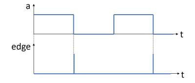
Write a program in Ladder Diagram that implements such edge recognition, without using the dedicated edge recognition contact. Assume that the variable a is initialized to 1.
