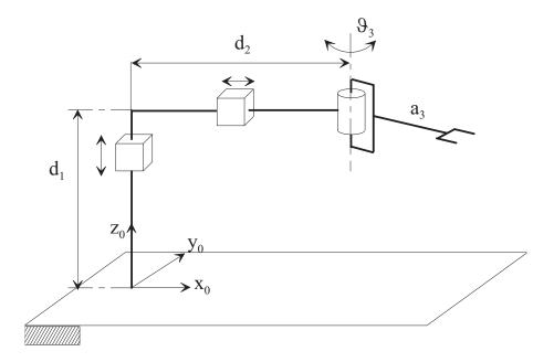
Find the expression of the direct kinematics of the robot, in terms of the position coordinates of the end effector with respect to the joint variables  $d_1$ ,  $d_2$ , and  $\vartheta_3$ .
