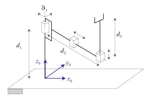
Find the expression of the direct kinematics of the robot, in terms of the position coordinates of the end effector with respect to the joint variables  $\vartheta_1$ ,  $d_2$ , and  $d_3$ .
