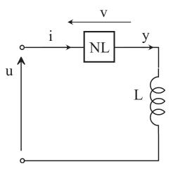
where the nonlinear element NL enforces the following relation between the current i passing through it and the corresponding voltage v across it:
