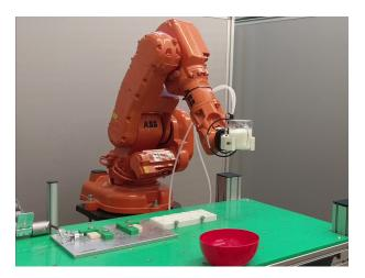
The robot should be moved in such a way to avoid spilling of the liquid from the container. In a first approximation, the sloshing dynamics of the liquid can be modelled with a pendulum, see the following picture:
