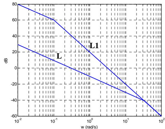
$$\varphi_c = -90^\circ - 2 \times \arctan(0.3) - \arctan(0.01) = -90^\circ - 2 \times 16.7^\circ - 0.5^\circ = -124^\circ$$
